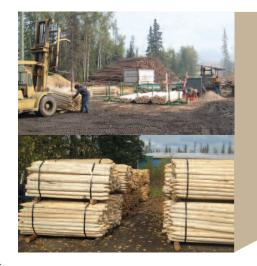
inches he can process and peel them to get good pine to make two to three inch, and three to four inch posts and railings, fencing, etc., some up to 16 feet long.
